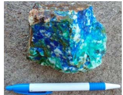
Rock sample from Gray's Vein – 8.26% Cu; 4.28g/t Au; 25oz/t Ag (Source: NiPlats)
